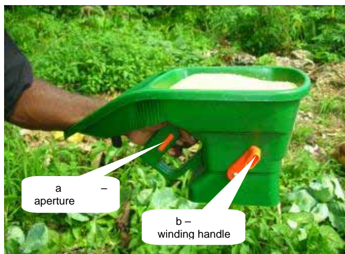
Figure 6. Image of a "Scott" bait spreader showing the winding handle (a), the aperture adjustment (b) and correct grip. Set the aperture at "1".
