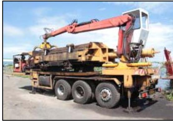
Figure 6. Mobile scrap metal compactor, CRT centre.
